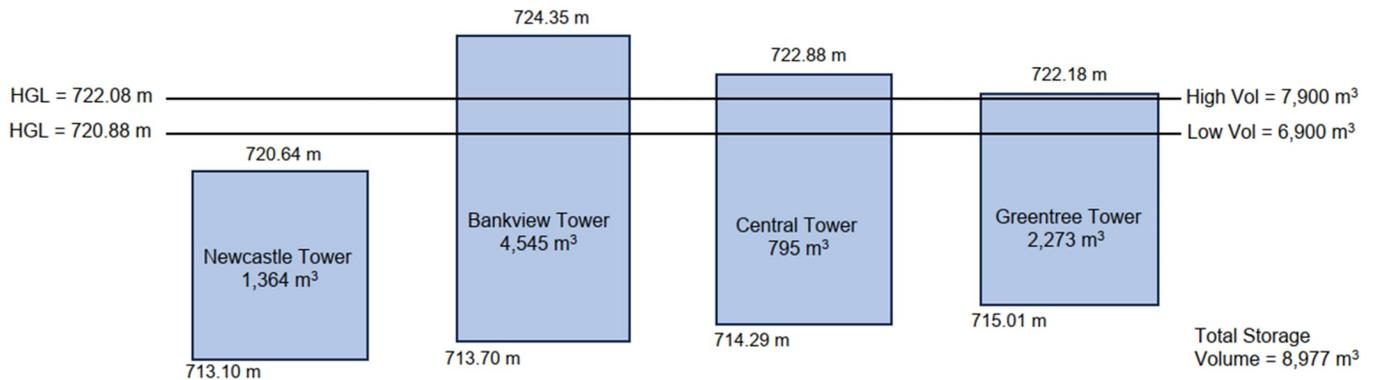
It was determined that the low volume of 6,900 m<sup>3</sup> was equivalent to an HGL of 720.88 m and the high volume of 7,900 m<sup>3</sup> was equivalent to an HGL of 722.08 m. The results were simplified to a pump start at 720.9 m HGL and stop at 722.1 m HGL. It is acknowledged that this is a simplification of the system and that individual water tower HGLs may vary minimally due to their location within the distribution system.
