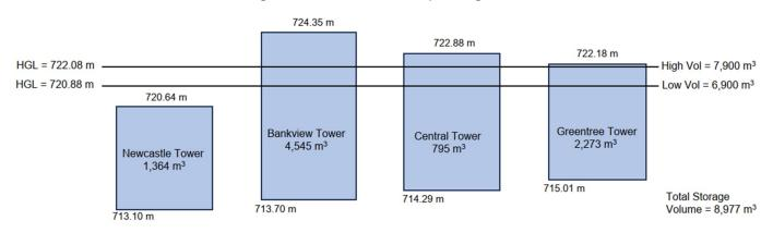
Figure 3-5 Water Tower Operating Levels
